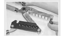
4 Lubricate your mold using Alox Beeswax Mix Bullet Lube [Lee #90007]. DO NOT USE Lee Liquid Alox as it will bake on the mold surface, preventing proper closure.
