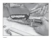
7 Quickly cut the sprue by moving the sprue lever to the right. The sprue can be dropped
