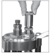
Thread assembly into powder through expanding die or rifle charging die. Make sure o-ring is located between the top of the powder through expanding die and the powder measure riser
