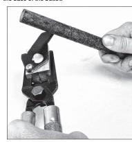
OPEN HANDLES and tap handle hinge bolt to shake bullet onto soft cloth. If mold doesn't open easily, gently tap the aluminum block near the bottom while applying light pressure to open the blocks.
