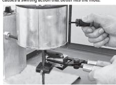
JUST BEFORE complete solidification of the metal in the sprue plate, strike the sprue plate with a wood dowel to cut the sprue. Move plate 90° to clear the base of the bullet.
