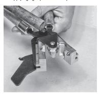
WARNING Do not strike core pin holder. If bullets do not drop free with a light tap on hinge bolt, heat corner of mold in molten metal
