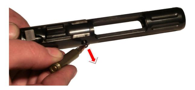
13. Grasp the bolt with the firing front tip facing up as shown on the picture below and by tapping the bolt let the firing pin slide out of the firing pin channel and remove the firing pin.
