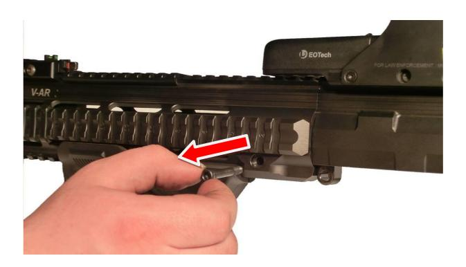
9. Pull the handguard in the direction towards the muzzle and remove it. If the handguard can't be initially pulled off the barrel nut, tap the rear edge of the side weaver rail using an appropriate tool such as a rubber mallet, piece of wood or a wooden hammer grip.
