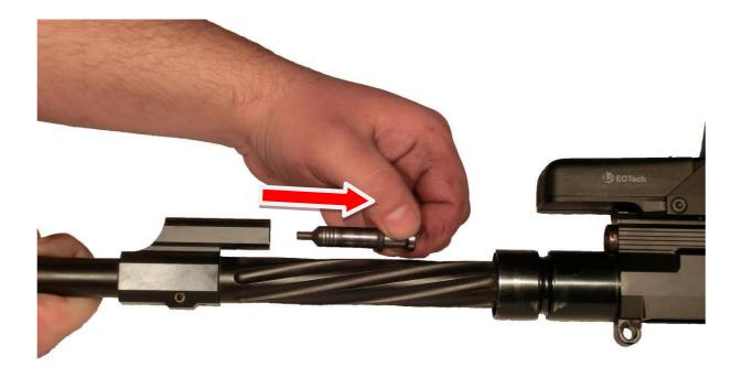
12. Using the tip of a cartridge bullet or other suitable tool remove the firing pin cotter pin from the bolt.
