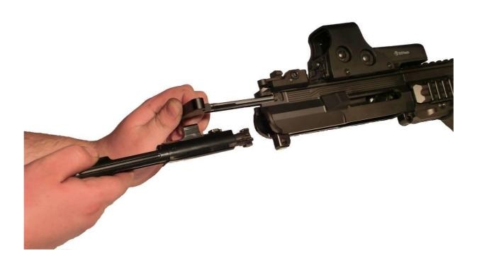
7. Grasp the charging handle and retract it all the way to the rear then pull it downwards and out of the receiver.
