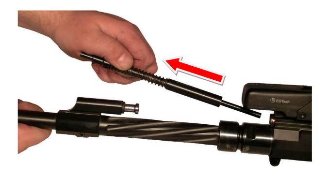
11. Grasp the piston and remove it from the piston cylinder by pulling it to the rear.
