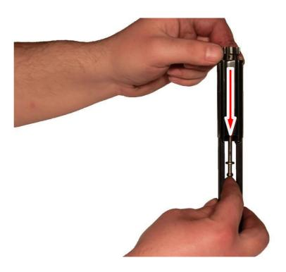
14. Grasp the bolt rotation driving pin and pull it out of the bolt.
