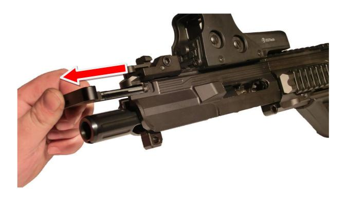
6. Grasp the rear part of the bolt and remove it from the receiver.
