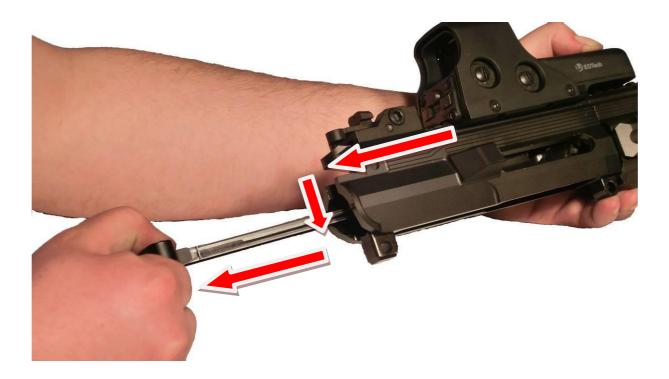
8. Using 4 mm Allen key remove the screw which tightens the handguard against the barrel nut by turning it counterclockwise. Remove the screw.
