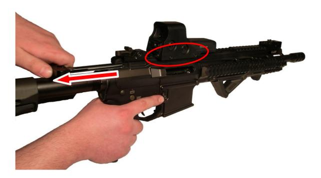
3. Using the tip of a cartridge, or other suitable tool, push the pins connecting the upper and the lower receiver inwards from the left side of the rifle. First the rear pin then the front pin.
