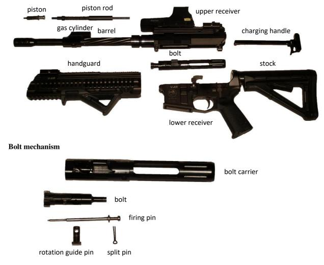
The 9 mm rifle has no gas cylinder, no piston and no piston rod. The bolt mechanism is comprised of bolt, firing pin and split pin only.
