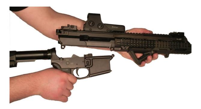
5. Pull the bolt out of the receiver by fully retracting the bolt charging handle.
