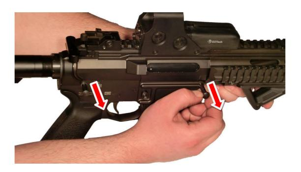
4. Disconnect the upper and the lower receiver. There is no need to further disassemble the lower receiver with the stock, pistol grip, magazine well and the trigger mechanism.
