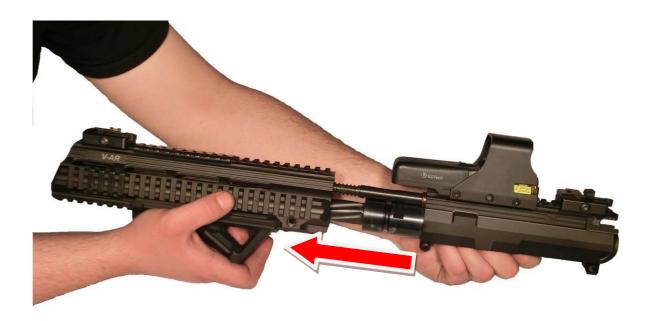
10. Grasp the piston rod and press its spring rearwards into the frame, then lift its front part and pull it out towards the muzzle. The charging handle must be removed or fully retracted into its rear position, otherwise the piston rod can't be lifted upwards!
