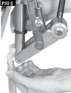
Slide retaining ring on to assembly.
