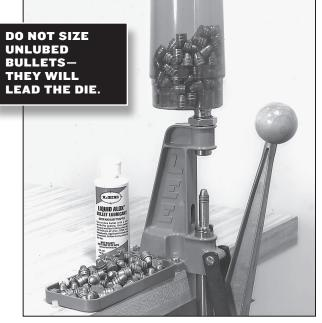
Very large and long bullets with a flat nose may stack and push the cover off the box. A washer under one edge of the press base will tilt the press sufficiently to prevent stacking.
